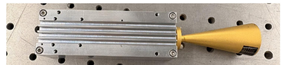
Fig. 1. Synthetic ECE validation for a DIII-D reference discharge (TRAVIS ray tracing): the simulated radiometer measurement (blue) reproduces the model electron temperature profile (red) over 85–108 GHz. Below: W-band on-chip receiver module with horn antenna, developed by UC Davis.
